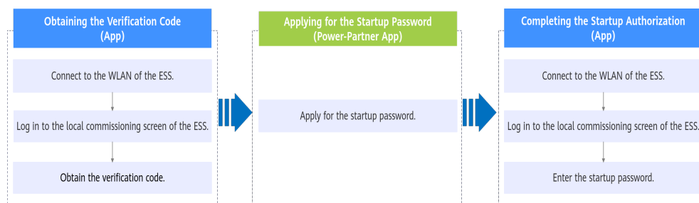
Figure 6-1 ESS startup authorization procedure
